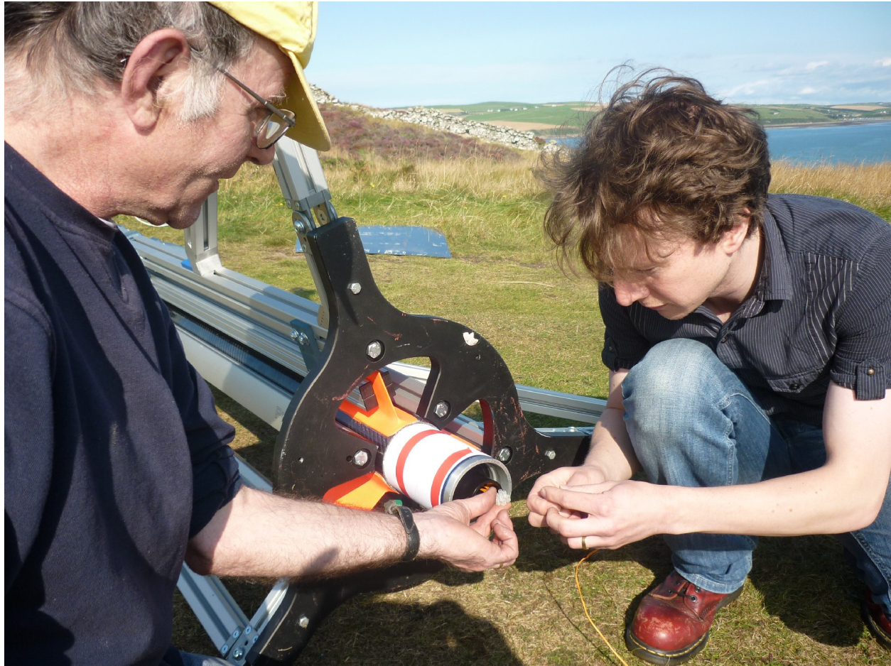
Figure 16. Connecting the launch controller to the 1 st stage.
